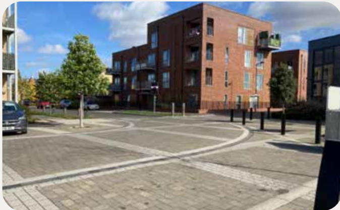
Figure 32. Public Space Materials Extend to Carriageway to Slow Down Vehicle Movements & Prioritise a Sense of Place
