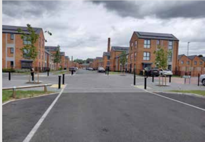
Figure 134. Tree Planting at a Junction to Give a Sense of Place and Reduce Vehicle Speeds, Leicester
